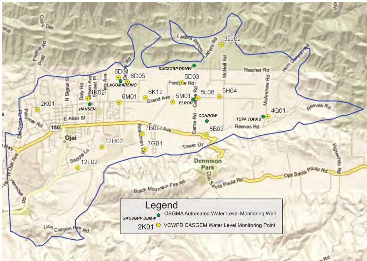
Figure 5: Locations of OBGMA Automated Water Level monitoring wells and VCWPD CASGEM Water Level Monitoring Wells. Note basin boundary is DWR 2003 delineation and has been superseded (Appendix E).
