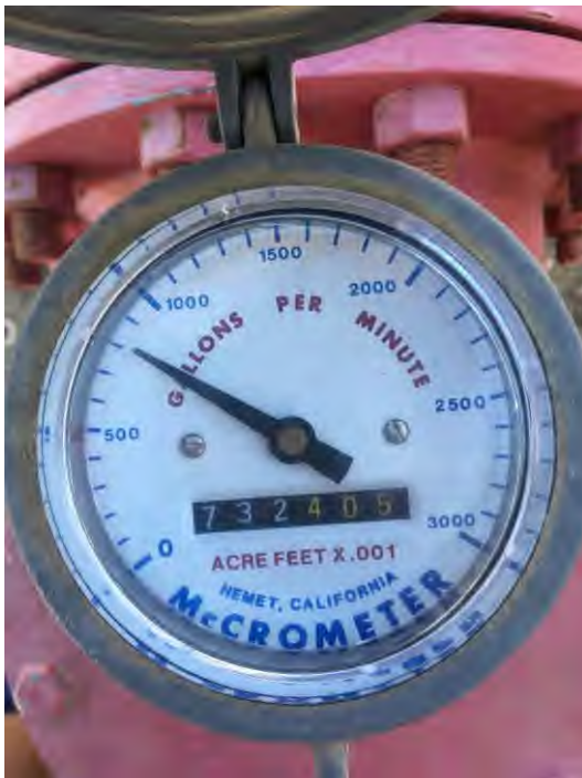
Figure 4: Three types of meters showing various means of accounting for extraction: Clockwise from top, 97720.1 gallons, 2949.1016 acre feet, and 732.405 acre feet
