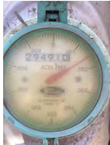
Figure 4: Three types of meters showing various means of accounting for extraction: Clockwise from top, 97720.1 gallons, 2949.1016 acre feet, and 732.405 acre feet
